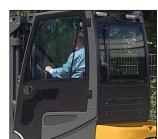
Raised operator cab (for special applications)
